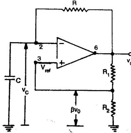
$$\text{Frequency, } f = \frac{1}{2R_f C \ln\left(\frac{2R_1 + R_2}{R_2}\right)}$$
