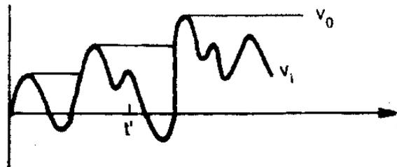
**Fig. 3.51 Output  $v_o$  corresponding to arbitrary input  $v_i$**
