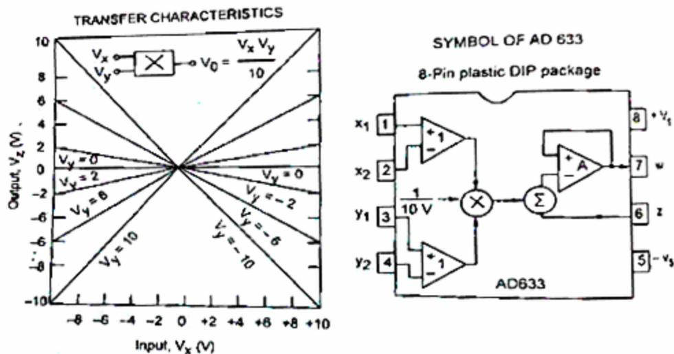
**Fig 40(b) Transfer characteristics**
