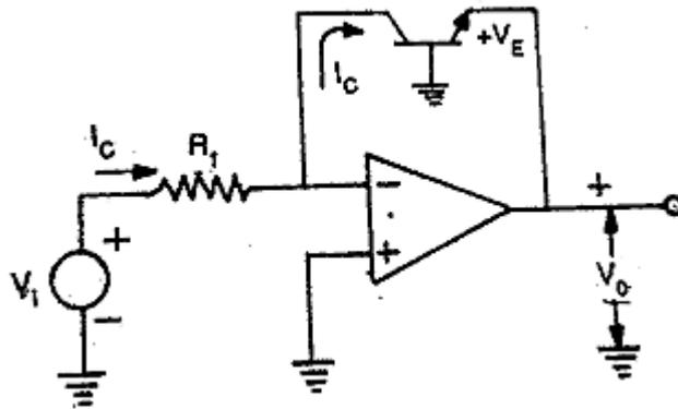
**Fig. 3.4 Fundamental log-amp circuit**
