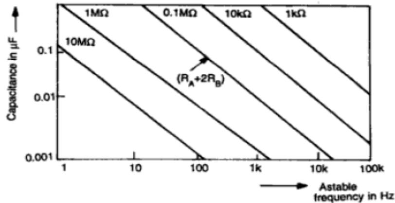
**Figure 18: Frequency dependence of  $R_A$ ,  $R_B$  and C**
