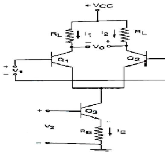
**Figure 37: Variable trans conductance amplifier**
