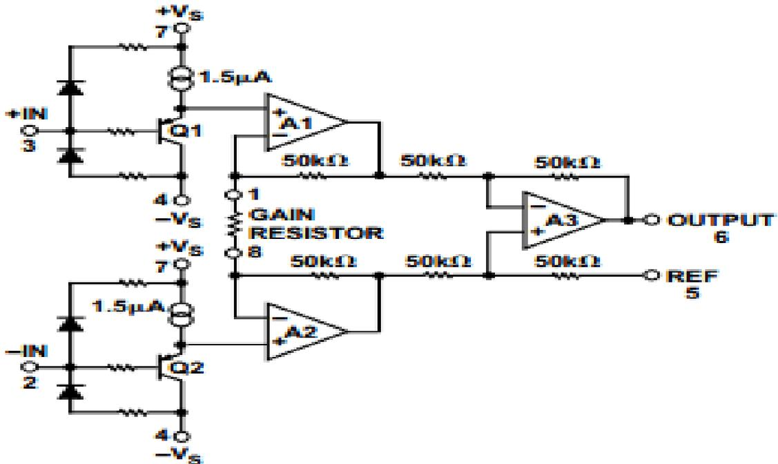
**Figure 1: AD623 Simplified Schematic**
