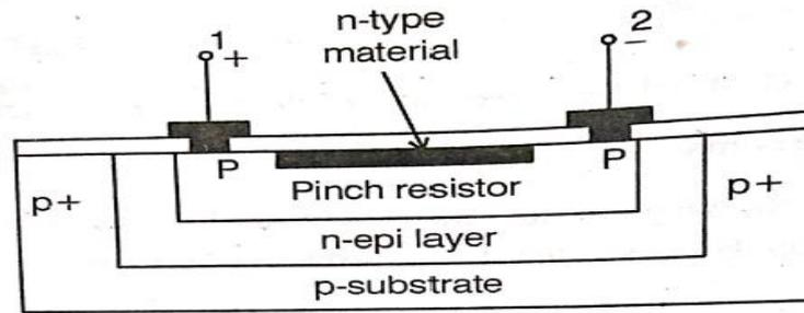
Fig 4.3.3 Pinched resistor
