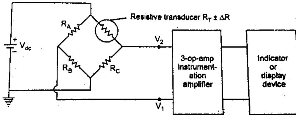
**Fig. 3.3 Instrumentation amplifier using Transducer Bridge**
