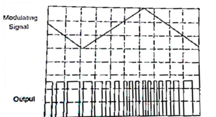
Figure 23: Pulse position modulator output
