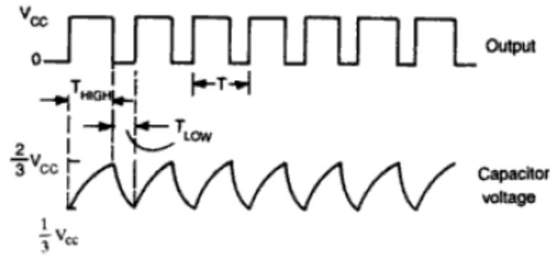
**Figure 17: Timing sequence of Astable multivibrator**
