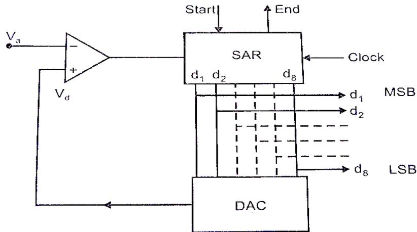
**Fig. 3.59 Functional diagram of Successive Approximation ADC**
