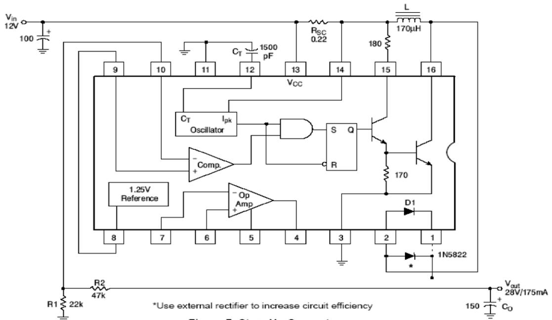
Figure 7. Step-Up Converter
