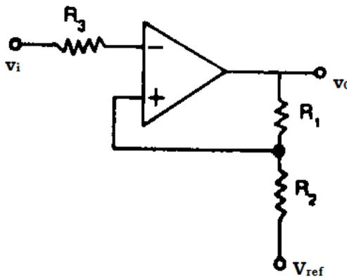
**Fig. 3.26 An inverting Schmitt trigger**
