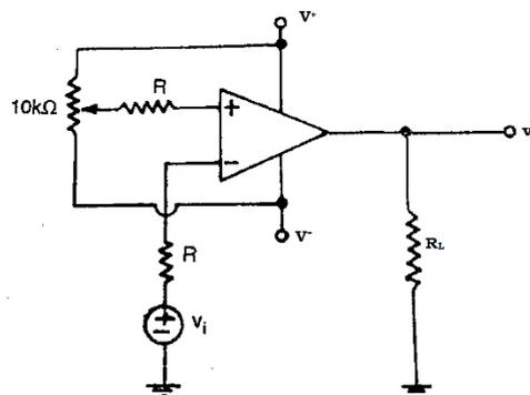
**Fig. 3.21 Inverting Comparator**
