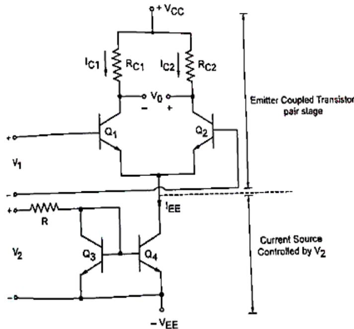
**Figure 34: Emitter coupled transistor**
