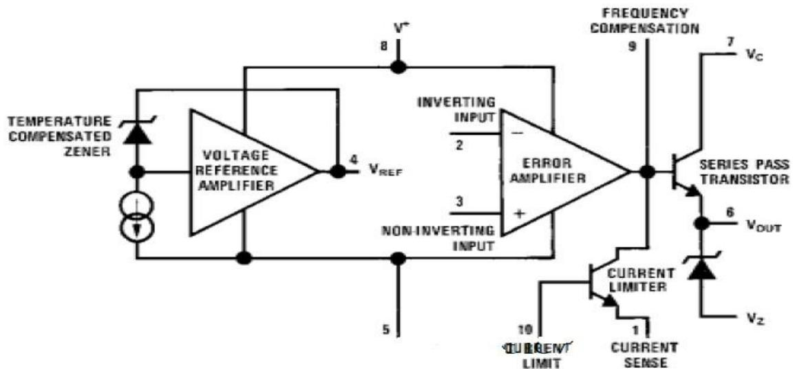
**Figure 8: Functional block diagram of IC723**
