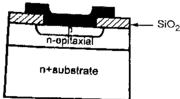
**13. Explain how a monolithic capacitor can be fabricated. (Dec – 14) (6)**
