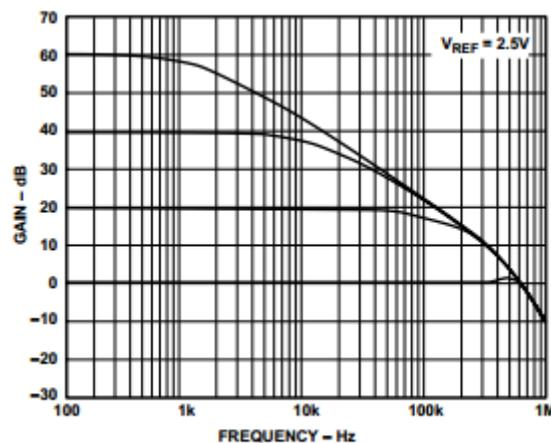
**Figure 2: AD623 Closed-Loop Gain vs. Frequency**
