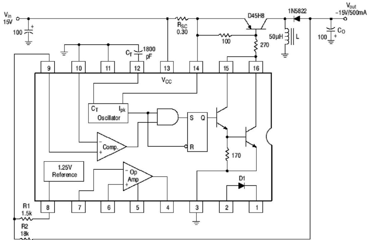
**Figure 17: Inverting switching regulator**
