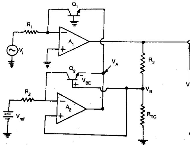
Fig. 3.6 Log-amp using two op-amps only
