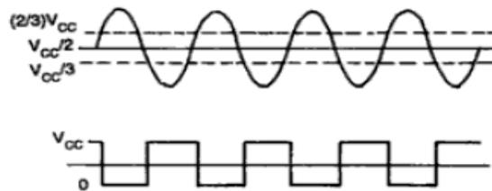
**Figure 25: Input Output waveforms of Schmitt Trigger**
