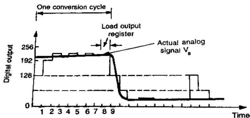
**Fig. 3.60 The D/A output voltage is seen to become successively closer to the actual analog input voltage**
