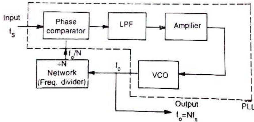
**Figure 29: Frequency multiplier using IC PLL**
