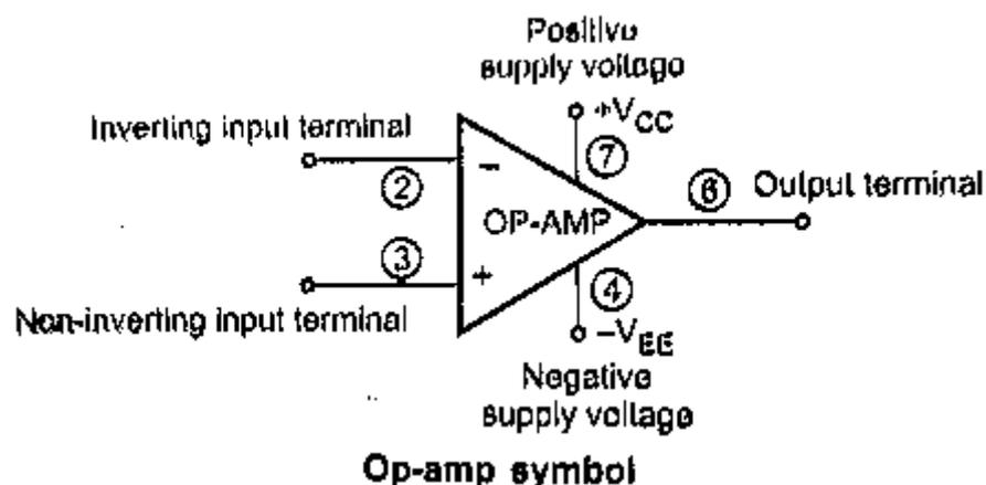
→ The op-amp is indicated basically by a triangle which points in the direction of the signal flow. All the op-amps have at least following five terminals:
