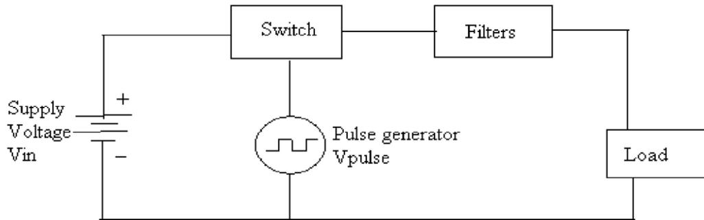
**Fig 12: Basic Switching regulator**
