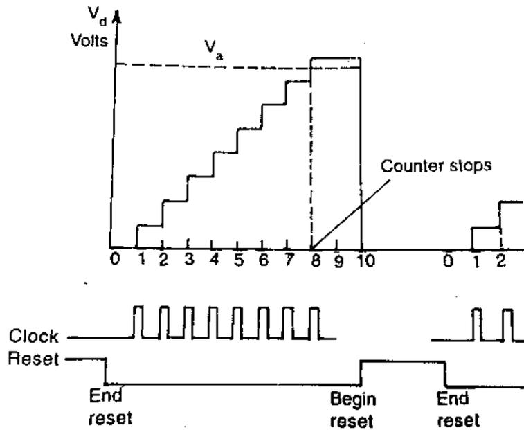
**Fig. 3.64 D/A output staircase waveform**
