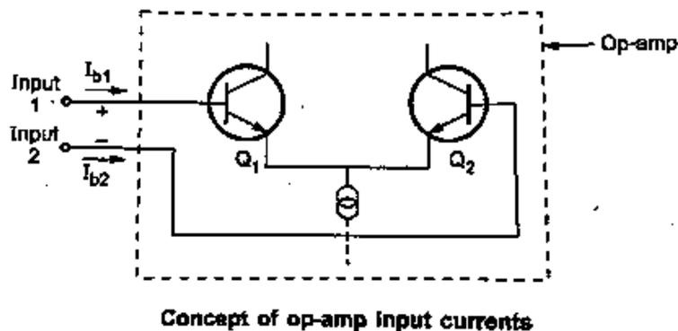
→ The algebraic difference between the currents flowing into the two input terminals of the op-amp is called **input offset current** and denoted as  $I_{ios}$ .
