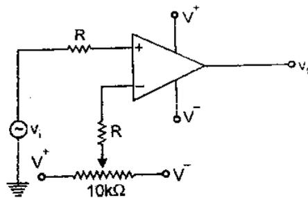
**Fig. 3.20 Practical Non-inverting comparator**
