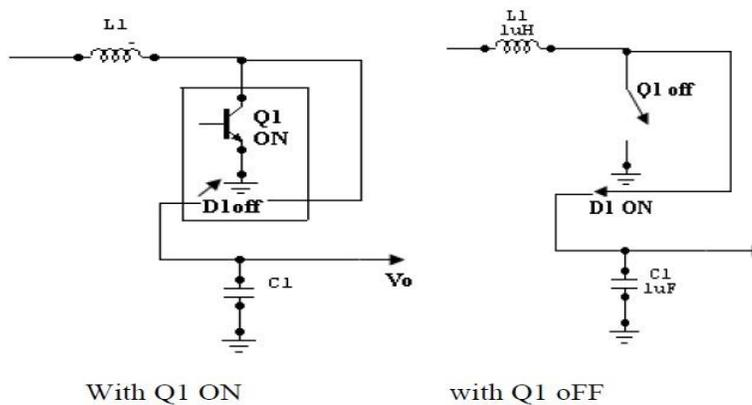
Figure 16: Step- up converter
