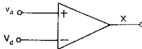
**Fig. 3.62 Comparator and its truth table**
