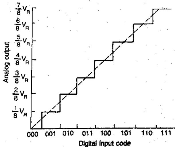
Fig. 3.57 Transfer characteristics of a 3-bit DAC
