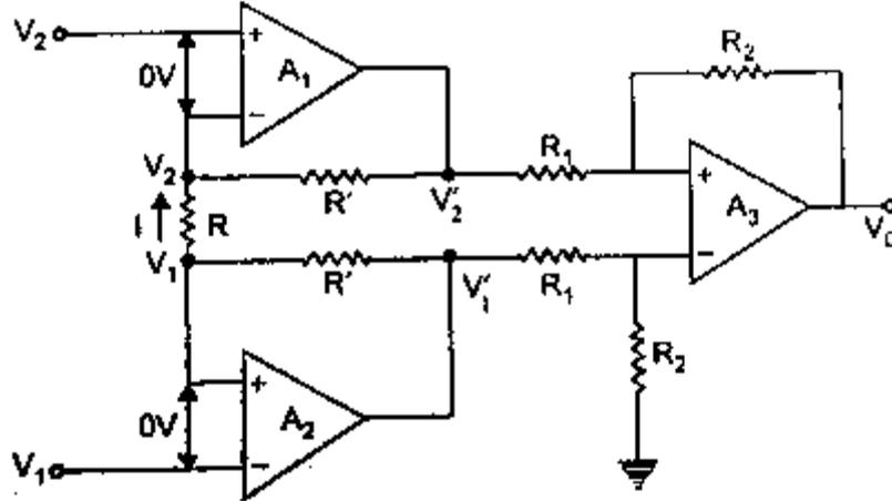
**Fig. 3.2 An improved Instrumentation amplifier**
