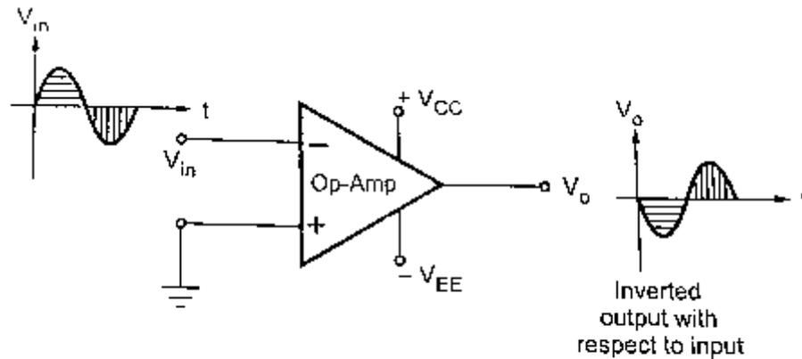
(a) Input applied to inverting terminal
