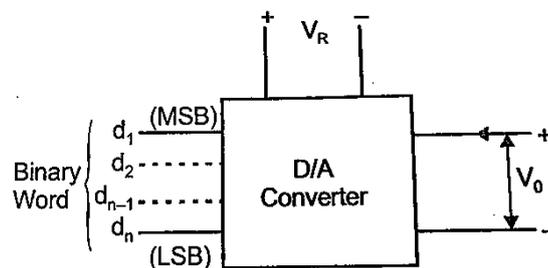
**Fig. 3.55 Schematic diagram of a DAC**
