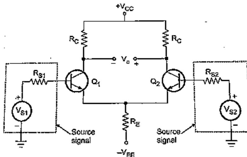
**Dual input, balanced output differential amplifier**
