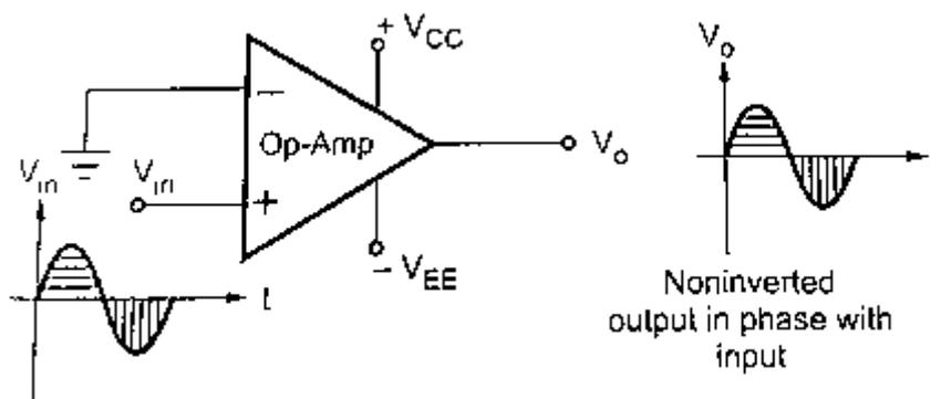
(b) Input applied to non-inverting terminal
