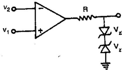
**Fig. 3.23 Comparator with zener diode at the output**
