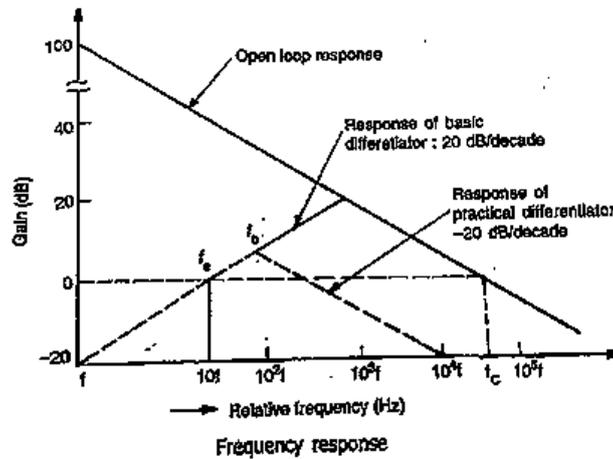
→ This 40 dB/decade change in gain is caused by  $R_1 C_1$  and  $R_f C_f$  factors.
