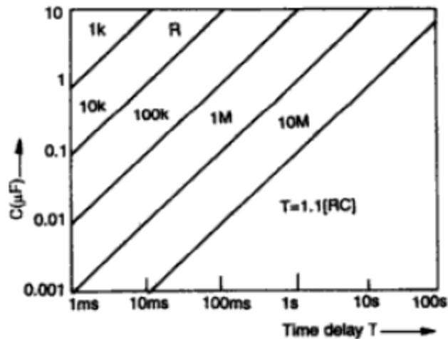
**Figure 6: Graph of RC combinations for different time delays**
