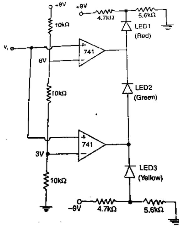
**Fig. 3.25 Three level comparator with LED indicator**
