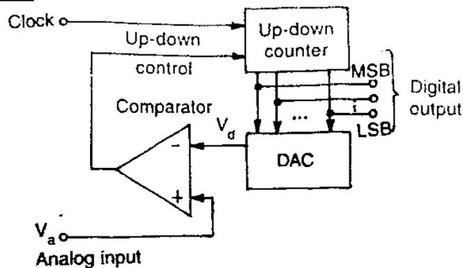
**Fig. 3.65 A Tracking A/D Converter**
