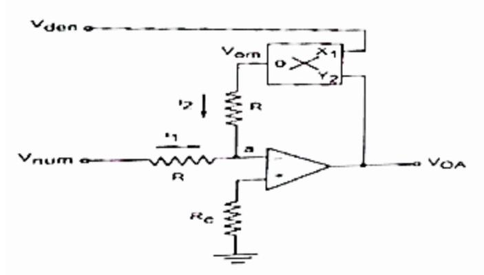
**Figure 43: Voltage divider**
