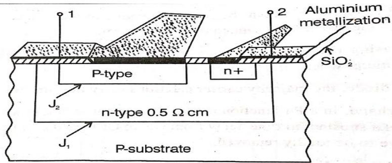
Fig 4.2.1 Junction capacitor
