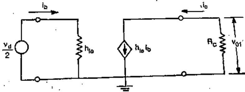
Small signal equivalent circuit of differential half circuit using  $h$ -parameter model
